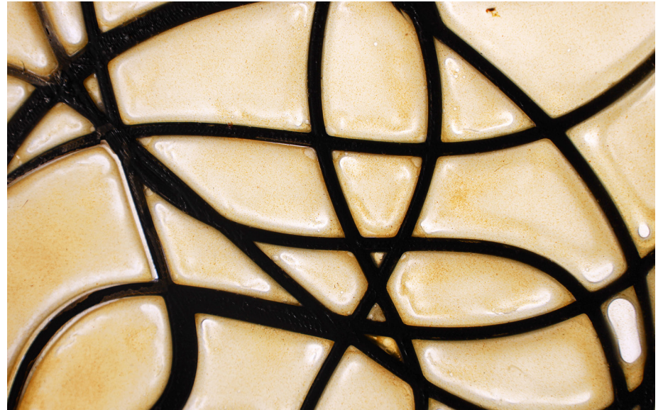
Elmers glue with liquid rust molded into a 3D printed PLA filament.
